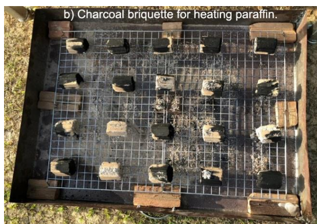
Fig. 6: Phase change heat storage system utilizing heat from charcoal briquette.
