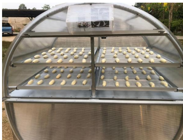
Fig. 5: Arrangement of ripe bananas inside the parabolic dome solar dryer.
