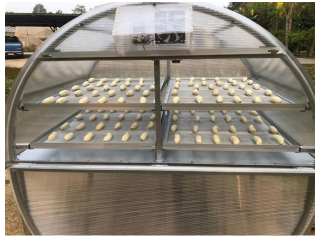
Fig. 5: Arrangement of ripe bananas inside the parabolic dome solar dryer.
