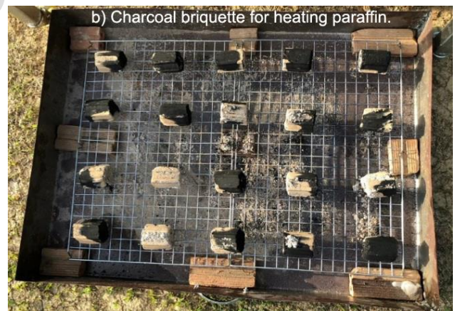
Fig. 6: Phase change heat storage system utilizing heat from charcoal briquette.
